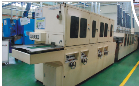
BRUSH & WASHING MACHINE LINE
